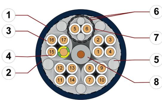
1. Outer jacket: Pressure extruded PUR mixture
