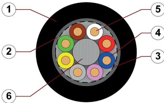
1. Outer jacket: Pressure extruded, oil-resistant PVC mixture
