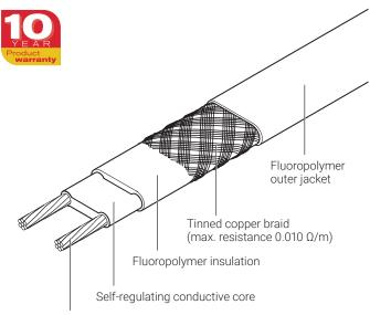
Electrical heat-tracing for process temperature maintenance applications up to 110°C which are not subject to steam cleaning.
