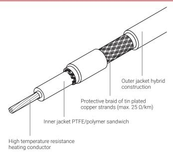
nVent RAYCHEM XPI-F is a polymer insulated (PI) series heating cable, suitable for use in ordinary and hazardous areas. It has been designed for freeze protection and low temperature maintenance applications on pipes, tanks and other equipment.
