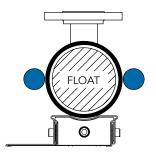
Probe mounting positions on Atlas<sup>™</sup>, Vector<sup>™</sup>, and Gemini<sup>™</sup> magnetic level indicators.
